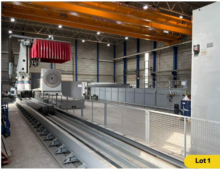
Lot 1: 2019 Valk Welding Panasonic TL-1800 Complete turnkey welding robot system
