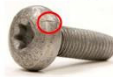
Sample side head crack on a fastener
